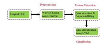
Figure 3: Block Diagram
