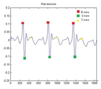
Figure 8: Detection of R, S and T Points
